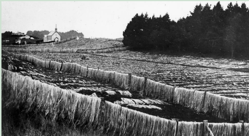
At Foxton, the flax leaves were scraped and washed to extract the fibres, which were then hung out to dry.
